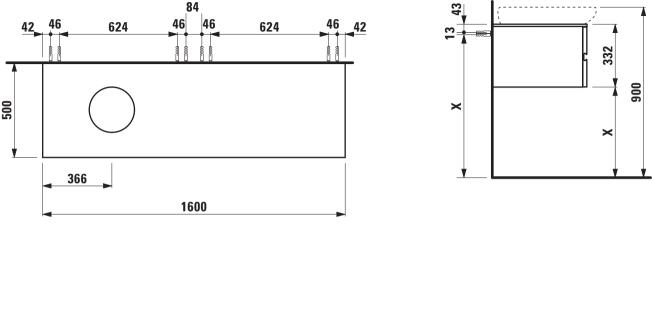
X = The exact hight must be set during installation.
