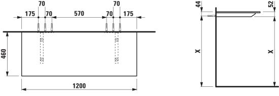
X = The exact hight must be set during installation.
