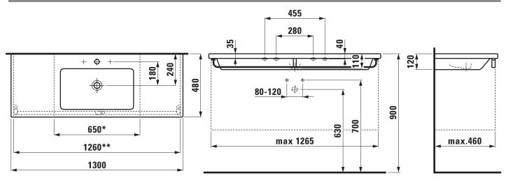
\* = minimum measure for cutting / \*\* = minimum measure for cutting with towel rail
