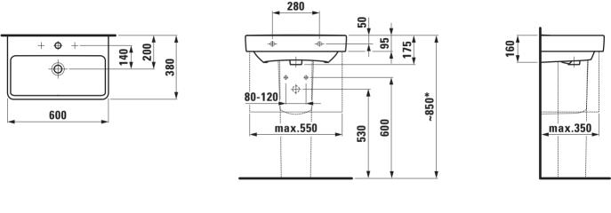
\* = Effective height must be fixed according to the height of the pedestal.
