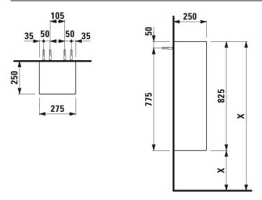
X = The exact hight must be set during installation.
