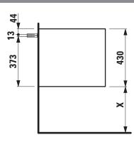
X =The exact hight must be set during installation.
